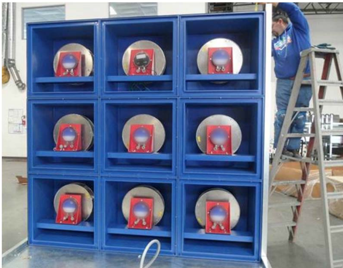
A 3x3 Multi Fan Unit designed to cool at 12,600 CFM
